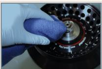
5.6.3.3 In the event of contamination caused by high-risk substances (bio hazardous or aggressive chemical reagents and radioactive reagents) wear a laboratory coat, gloves and goggles. If there is broken glass: Retrieve the bigger broken glass with forceps, remove small and powder shards with a damp lint-free cloth. Absorb blood with gauze or paper towel and subsequently, seal the material in a biohazard bag for safe disposal. Wipe the contaminated parts with Klercide 70/30
